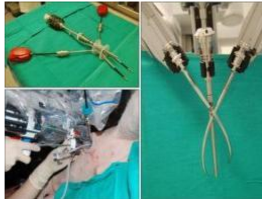
Intuitive Surgical's robotic instrumentation for single-site surgery (VeSPA)
