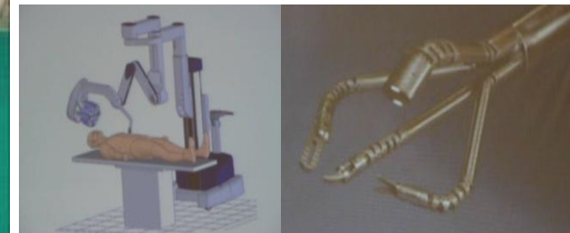
Intuitive Surgical prototype for single-hole surgery. (left) single robotic arm, (right) articulated end-effectors
