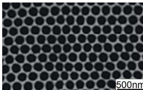
Fig. 1. SEM plan view image of hexagonally arranged macropores fabricated on Si using pre-patterning through a PAA masking layer. Pore diameter is \sim 180\text{ nm} and the lattice constant 200 nm.
