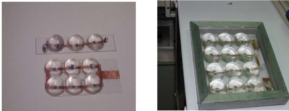
Fig. 5. Modules (left) and a panel (right) made of miniature concentration Si cells.
