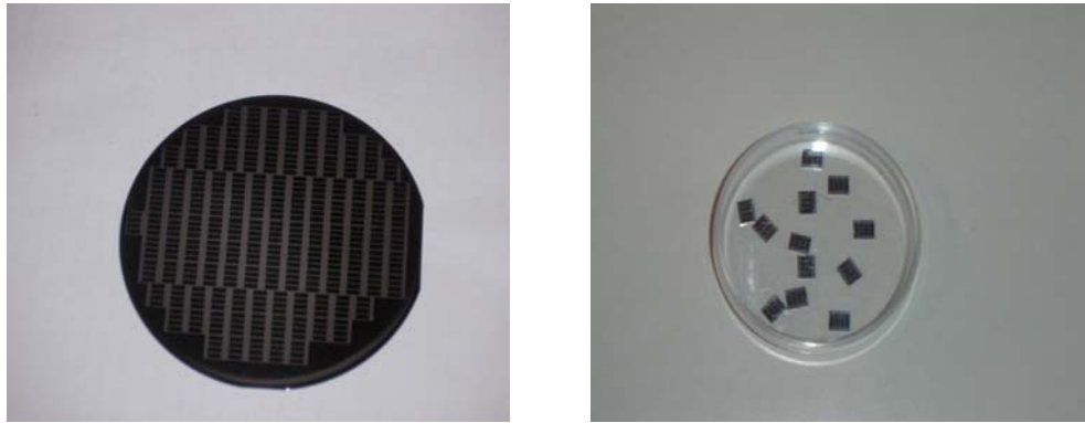
Fig. 4. Miniature PV Silicon cells with dimensions of 0,15 (0,5 \times 0,3) \text{ cm}^2 before (left) and after cutting (right).
