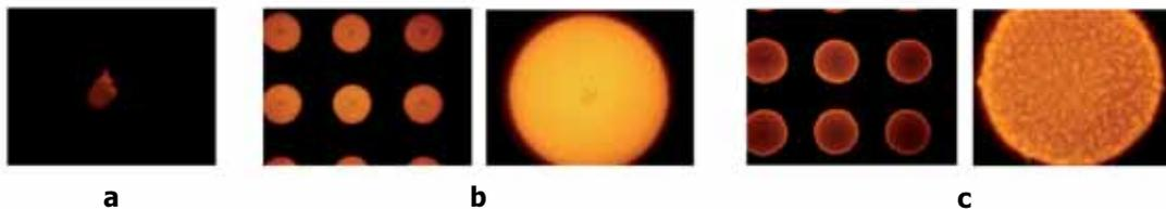
**Fig. 9:** Spotting of b-BSA on fresh SF<sub>6</sub> treated surfaces with a nanoplotter. Fluorescence images of spots of 200 µg/ml b-BSA (a) on an untreated PDMS surface, (b) on a 6 min SF<sub>6</sub> treated PDMS surface and (c) on a 20 min SF<sub>6</sub> treated PDMS surface.
