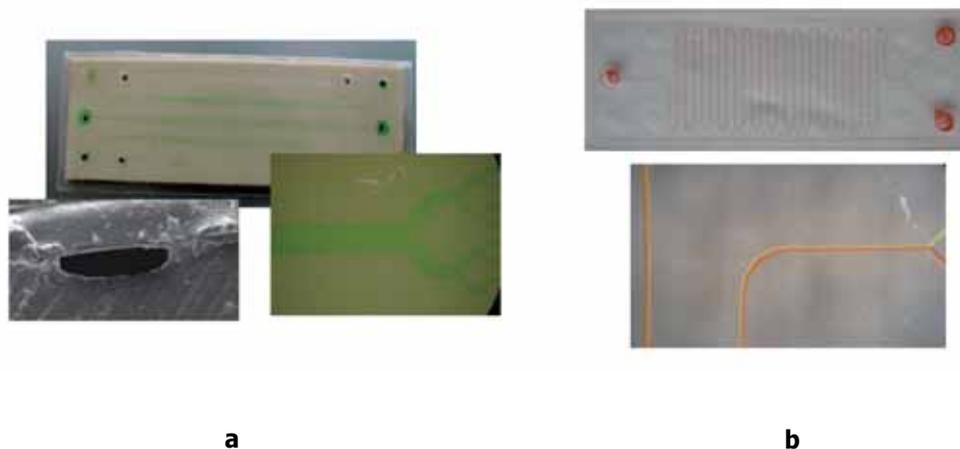
**Fig. 4:** **(a)** The microfluidic channel of PEEK and details in SEM of the cross section after the sealing. **(b)** Mixing of two liquids in PMMA plasma etched microfluidic mixer.
