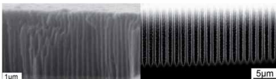
Fig. 12: Cross-sectional SEM images of macroporous Si fabricated by electrochemical etching of pre-patterned Si surfaces as follows: (a) Etching of a p + -type substrate in HF:ethanol 4:6 solution in volume. (b) Etching of a p-type substrates by electrochemical dissolution in an HF:DMF solution 12:88 in volume.
