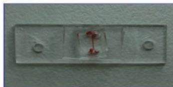
Fig. I.2.5: 100 \mu\text{m} deep PDMS microchannels fabricated with soft lithography and irreversibly bonded on a PMMA plate.
