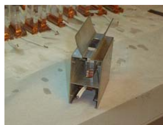
Fig. I.4.8: (Left) Photo of an encapsulated concentration solar cell. A prism ensuring the even distribution of energy on its surface and the current leads are integrated on the encapsulation. (Right) Photo of a cell ready to be positioned on PROTEAS.
