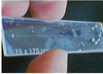
Fig. I.2.3: Microfluidic channel made on PMMA by means of direct plasma etching. Patterning and surface properties control are performed simultaneously.
