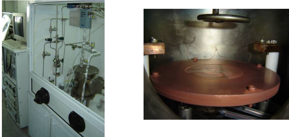
Fig. I.4.3: MOCVD system developed in 2005. Left, a view of the MOCVD system. The electronics, the DLI system and the stainless steel reactor are shown. On the right, a photo of the interior of the reactor is shown. The ring-like injector, the W filament and the substrate are distinguished.
