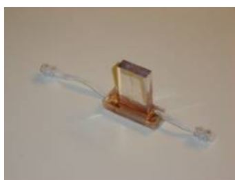
Fig. I.4.8: (Left) Photo of an encapsulated concentration solar cell. A prism ensuring the even distribution of energy on its surface and the current leads are integrated on the encapsulation. (Right) Photo of a cell ready to be positioned on PROTEAS.
