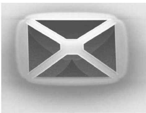
Fig. III.1.6: Fully released porous silicon micro-hotplate used as test structure for the stress measurement. The thickness of the membrane is 4 \mu\text{m} .
